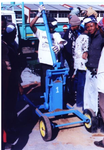
Figure 4 Training of a group in the production of cement stabilised compressed earth blocks (CEB) in Bankhara Bodulong.
