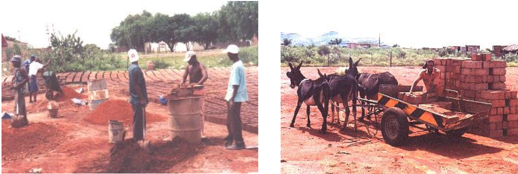
Figure 1 Local small scale brickyard and transportation of blocks to a building site in Bankhara Bodulong near Kuruman
