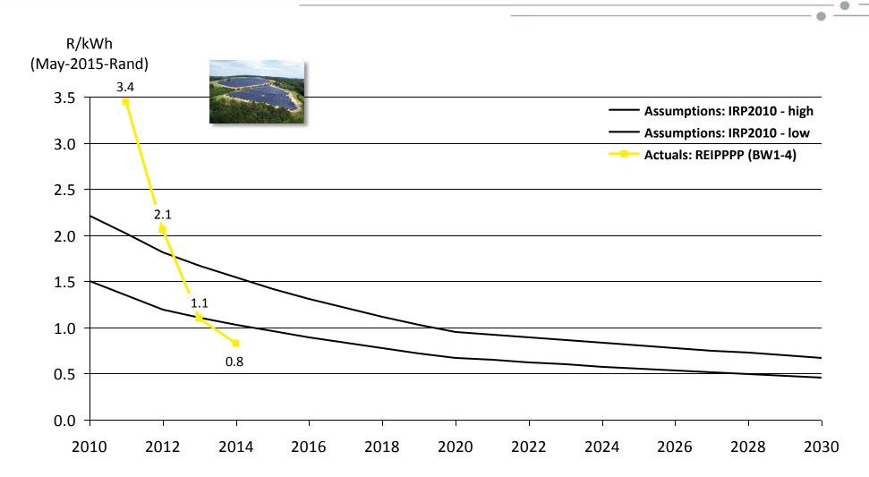
Assumptions: CPI used for normalisation to May-2015-Rand; LCOE calculated for IRP with 8% discount rate (real), 25 yrs lifetime, cost and load factor assumptions as per relevant IRP document; "IRP Tariff" then calculated assuming 80% of total project costs to be EPC costs, i.e. divide the LCOE by 0.8 to derive at the "IRP Tariff" Sources: IRP 2010; IRP Update; http://www.ipprenewables.co.za/gong/widget/file/download/id/279; CSIR Energy Centre analysis
