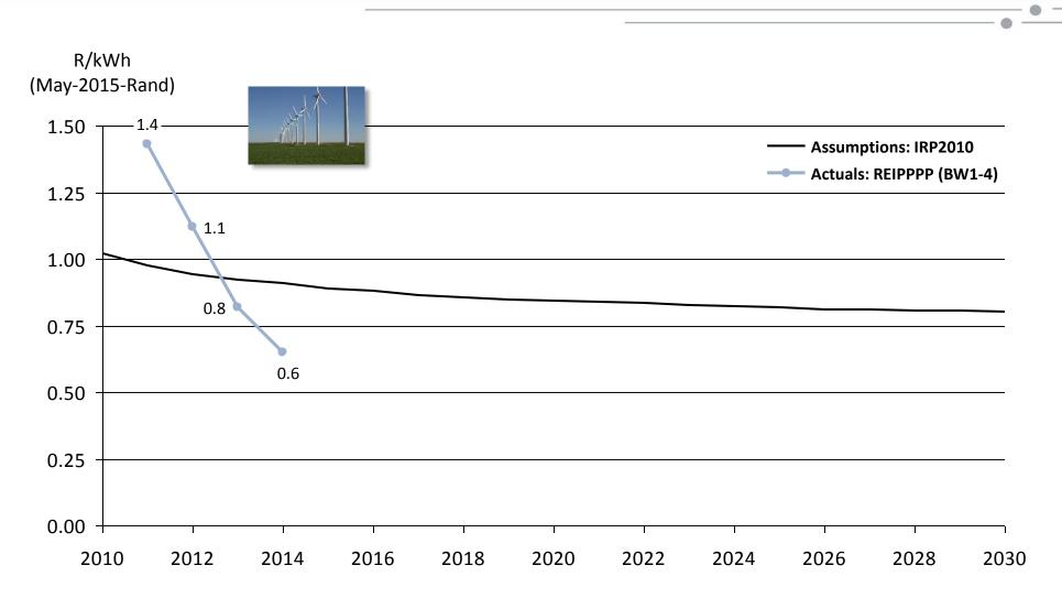
Assumptions: CPI used for normalisation to May-2015-Rand; LCOE calculated for IRP with 8% discount rate (real), 20 yrs lifetime, cost and load factor assumptions as per relevant IRP document; "IRP Tariff" then calculated assuming 80% of total project costs to be EPC costs, i.e. divide the LCOE by 0.8 to derive at the "IRP Tariff" Sources: IRP 2010; IRP Update; http://www.ipprenewables.co.za/gong/widget/file/download/id/279; CSIR Energy Centre analysis
