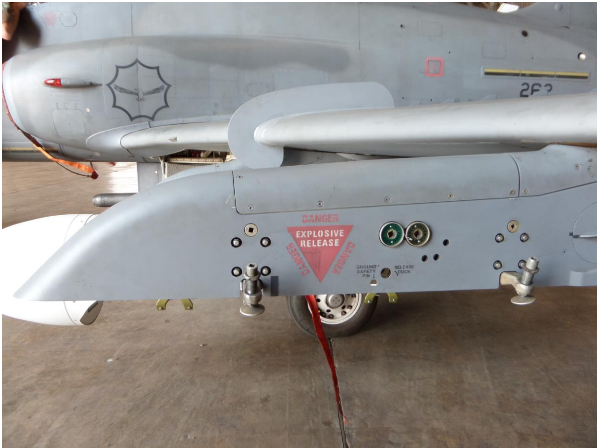
Figure 6: The ERU on the Hawk's outboard pylon (the ERU on the centerline pylon is identical)
