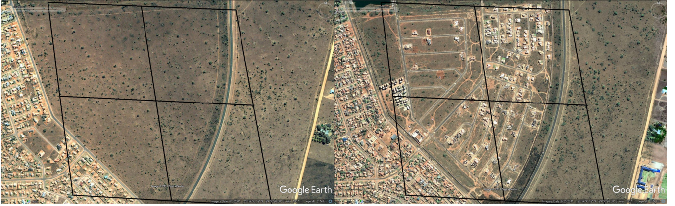
Figure 6. Land cover change detected in the suburb of Polokwane Extension 28 ( 23^{\circ}54'31.41''\text{S} , 29^{\circ}30'24.80''\text{E} ) located in the Limpopo province, South Africa. The Quickbird image on the left was taken on 3 June 2001 and on the right on 25 September 2011 (Courtesy of Google TM Earth). Only the top right MODIS pixel was flagged as changed. The three remaining pixels had to little change in the geographic footprint to be detected.
