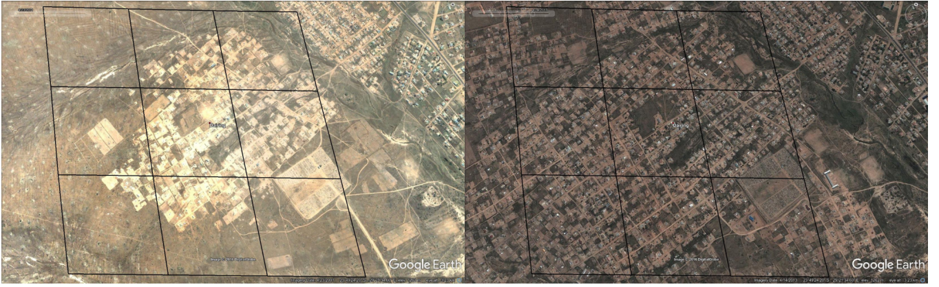
Figure 5. Land cover change detected in the town of Dairing ( 23^{\circ}49'22.73''S , 29^{\circ}21'27.55''E ) located in the Limpopo province, South Africa. The Quickbird image on the left was taken on 23 April 2001 and on the right on 14 April 2013 (Courtesy of Google TM Earth). This detection was made on a small existing settlement growing borders and internal increase in dwellings. All these pixels were successfully detected by our method.
