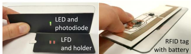
Figure 4: Standalone color detector design with printed wireless RFID module included.
