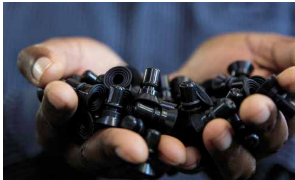
Rubber suction pads for the nose clips shortly after having been removed from the manufacturing mould.
