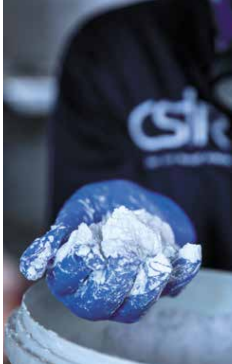
Synthetic hydrotalcite nanoclay produced by Greenfield Additives at the CSIR.
