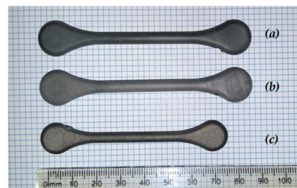
Figure 2—Standard MIM 'dogbone' component as observed during MIM processing – (a) as-moulded, (b) solvent-debound and (c) sintered at 1300°C
