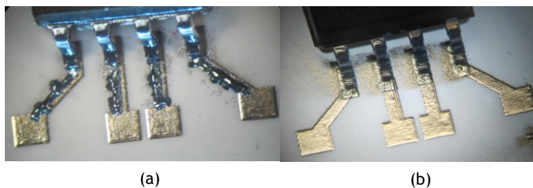
Figure 8. Inkjet printed pin connections using (a) 5 \mu\text{m} drop spacing with 1 layer and (b) 35 \mu\text{m} drop spacing for 3 layers.
