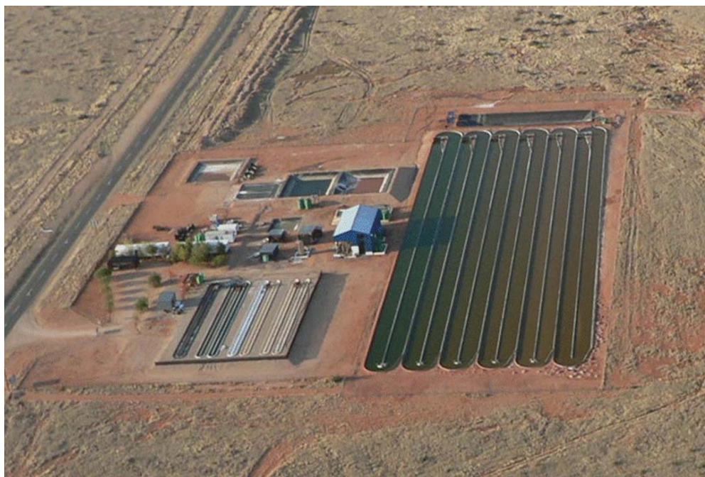
Figure 3: Aerial view of open raceway ponds used for the production of \beta -carotene near Uppington, South Africa
