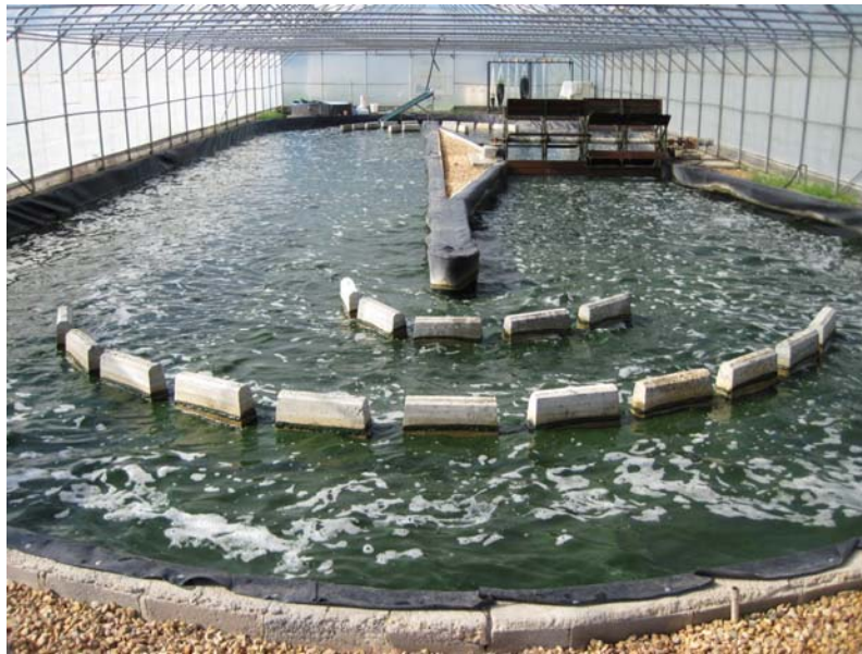
Figure 2: Spirulina being cultivated in a raceway pond
