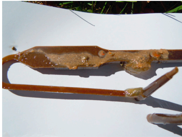
f0010 Fig. 7.1 Biological development on the surface of Flax/PLA biocomposite.
