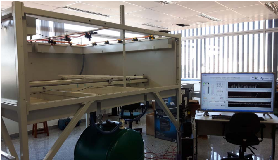
Fig. 10.2. Front view of the development system for projects dedicated to the application of liquid agricultural inputs based on the advanced sensors-based platform. In the background is the panel with electrical, electronic and hydraulic components and the front boom sections with the nozzles and spray tips.
