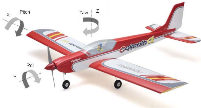
Fig. 18.1. Angular movement and directional movement.
