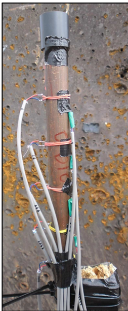
Figure 4: The Cu tube with light sensors and ionisation probes
