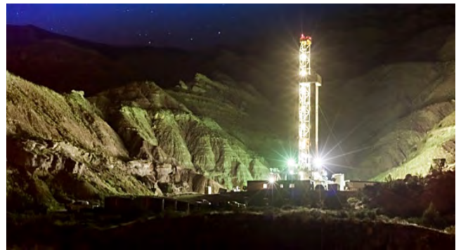
Figure 14.5: Wellpad with drilling rig at night (processingmagazine.com)
