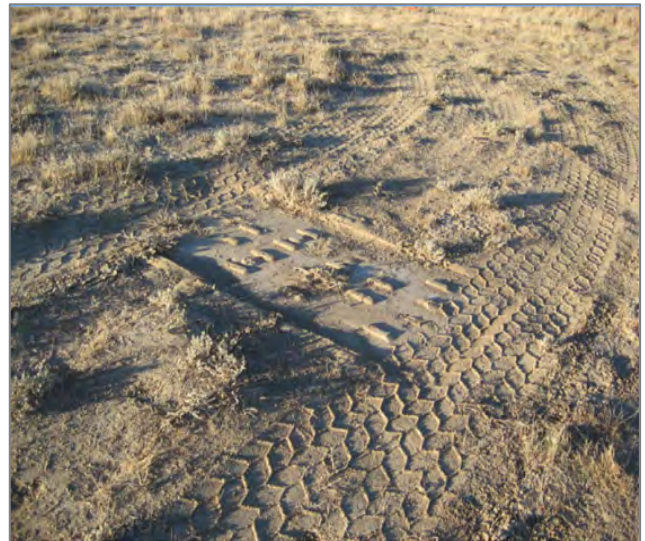
Figure 1.21: Ground impression left by the vibrator pad of a vibroseis truck (Source: Shell).
