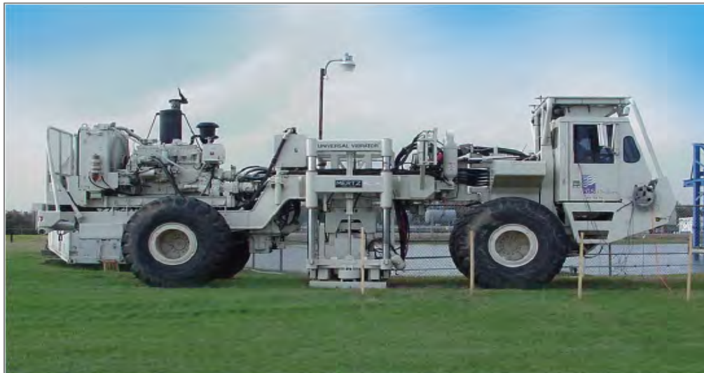
Figure 1.20: Seismic vibration (vibroseis) truck ( Source: Shell ).
