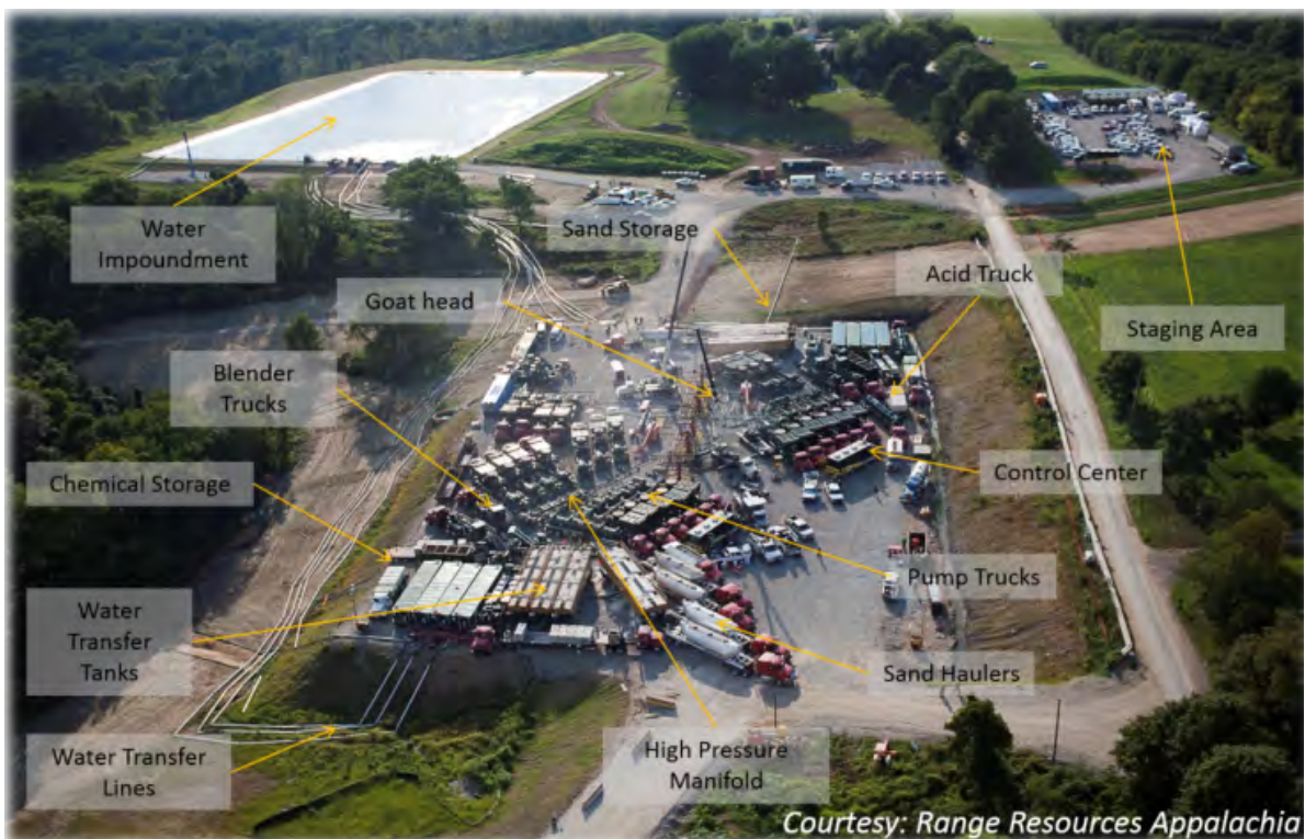
Figure SPM 1.6: Production wellpad with supporting infrastructure in the United States (see annotations). In terms of current South African legislation, open water storage (impoundment) such as illustrated in this example from North America, would not be permitted. Image sourced from Range Resources Corporation.
