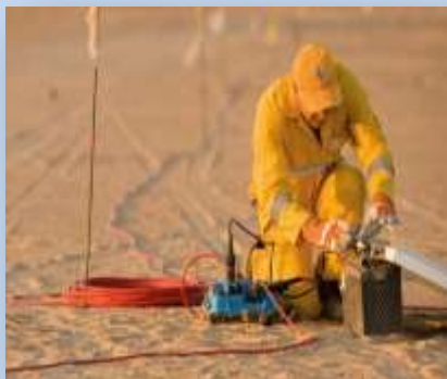
Personnel setting up a seismic data collection system which includes a small recording box, a battery, and an array of geophones. Fibre optic cables laid out in a grid pattern over the survey area transmit the signal from the recording box to the recording truck (Source: Shell).
