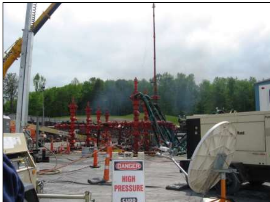
Figure 1.30: Example of a fracking operation underway, involving a series of wellheads (Source: Tom Murphy (n.d.), Pennsylvania State University, USA).
