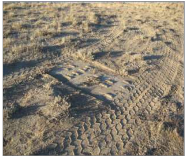
Figure 1.21: Ground impression left by the vibrator pad of a vibroseis truck (Source: Shell).
