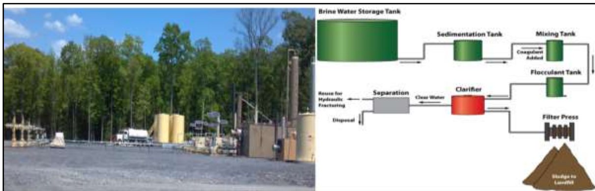
Figure 1.31: Schematic illustration of a produced fluid management system (Source: Tom Murphy (n.d.), Pennsylvania State University, USA).
