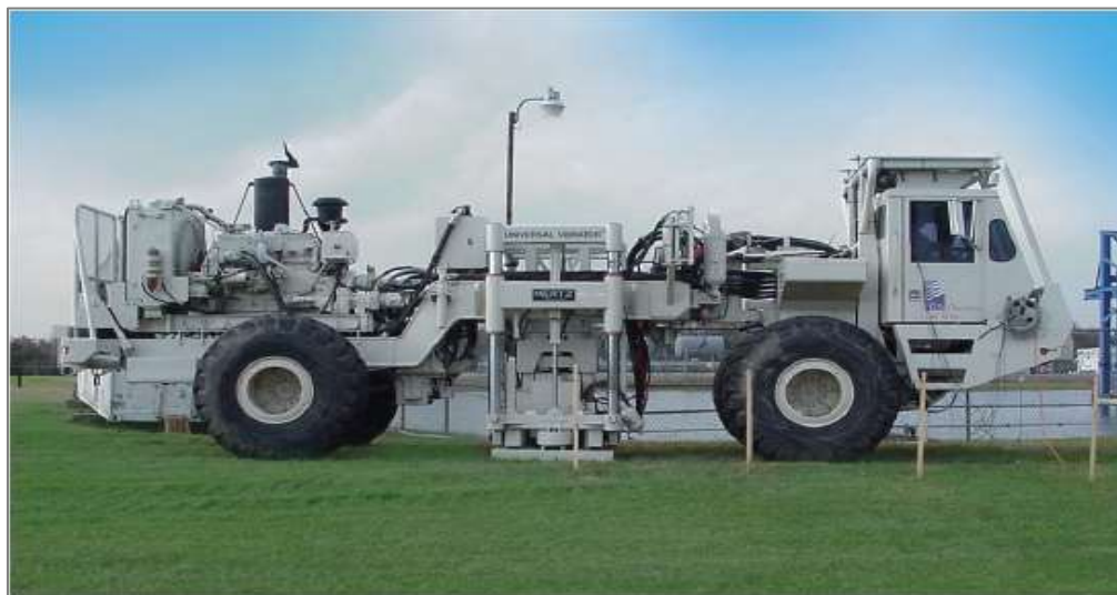
Figure 1.20: Seismic vibration (vibroseis) truck ( Source: Shell ).
