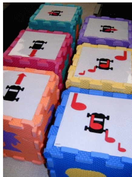
Figure 2. The six instructions used in the tangible programming system (clockwise from bottom left): move forwards, move back, turn left, turn right, play tune number one, and play tune number two.
