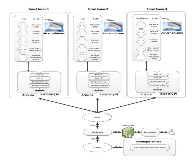
The experimental room consists of the following sensors, as well as an actuator.
