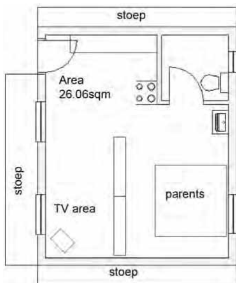
Figure 23.4: Lack of privacy: toilet in small house
