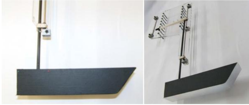
Fig. 8 The Hull mounted to the Balance
