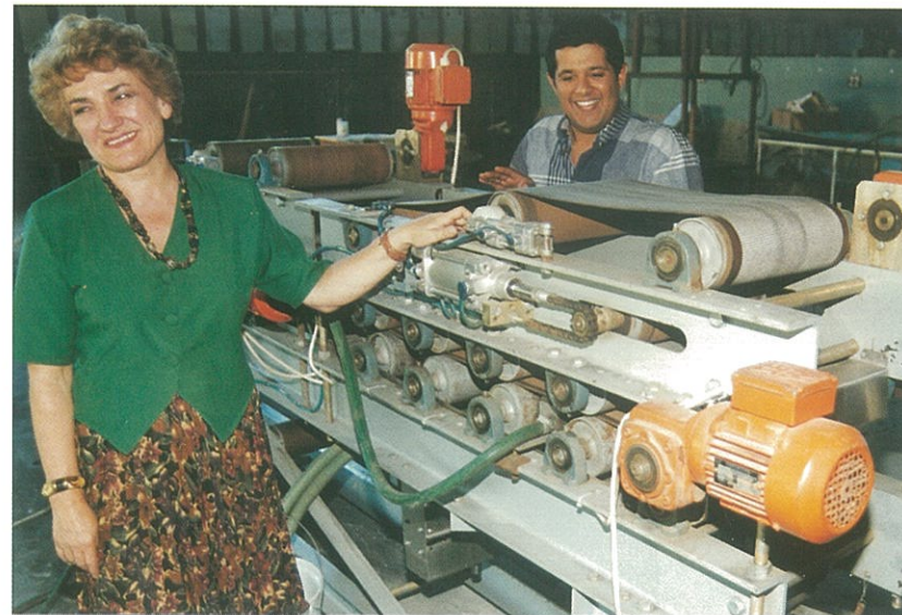
Electro-osmotic belt filter method of sludge disposal
