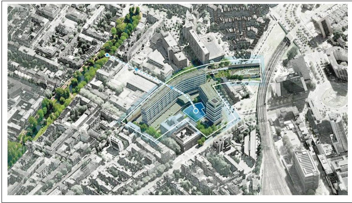
Figure 2: De Urbanisten's Watersquare Project in Rotterdam is a sunken plaza that doubles as a catchment system to manage stormwater (Gendall 2013).
