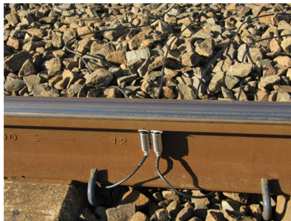
Figure 3 Four transducer array (two transducers hidden on opposite side of rail head)
