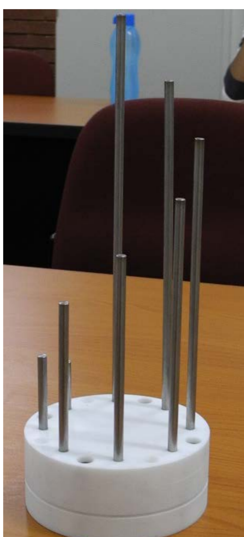
Figure 3 | Photograph of mechanical deflection sensor
