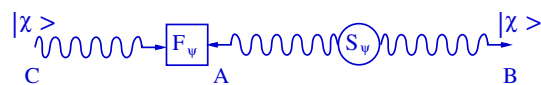
Figure 2 | Teleportation using a filter: source S_\Psi produces a pair of systems A and B in state |\Psi\rangle . System A and system C are to be projected by a filter F_\Psi into state |\Psi\rangle . If successful, the filtering transfers the initial state of C to system B .
