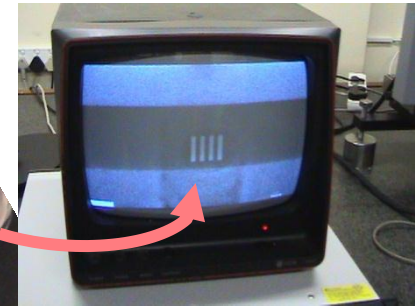
Four-bar target imaged by infrared camera
