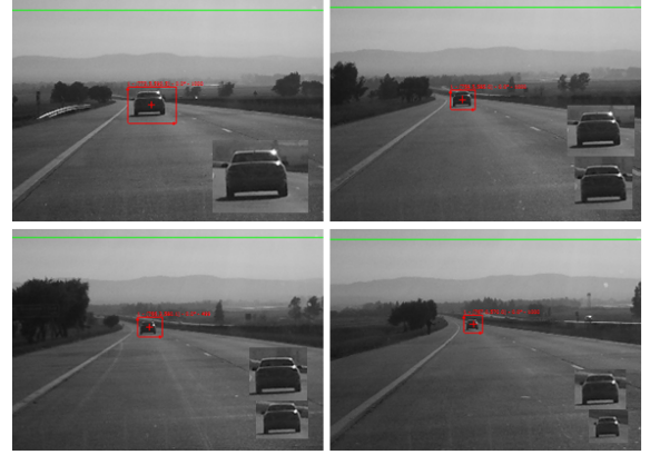
Fig. 3. Demonstration of how the lane width, at the point where the vehicle meets the road, is inversely proportional to the headway distance. This Figure also shows how multiple templates were detected.
