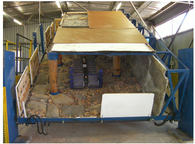
Fig. 2. The MSP robot navigating the stope at a 28^\circ angle
