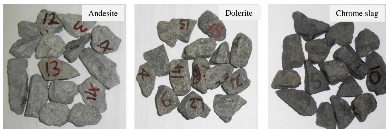
FIGURE 2 Example of aggregate particles scanned for this study.
