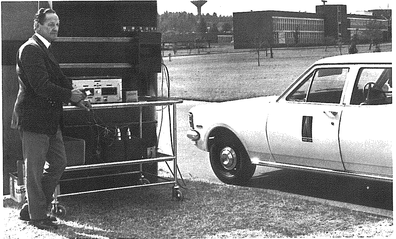
Pedestrians are involved in traffic accidents for various reasons, amongst others defective judgement of the velocity of an approaching vehicle. This apparatus is used in road safety research to determine the ability of pedestrians to estimate the velocity of approaching vehicles.
