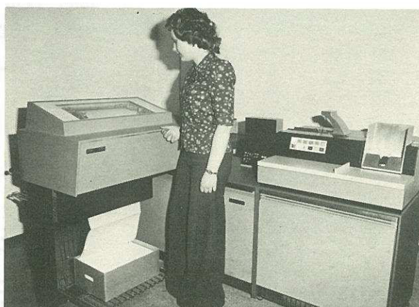
A high-speed computer terminal which permits remote entry and retrieval of batch jobs.
