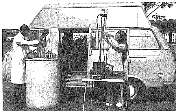
A mobile laboratory used by the APRG to measure pollutants in the atmosphere. On the left a sample of air is collected in a special container for analysis. On the right particulate material is collected in an electrostatic precipitator.
