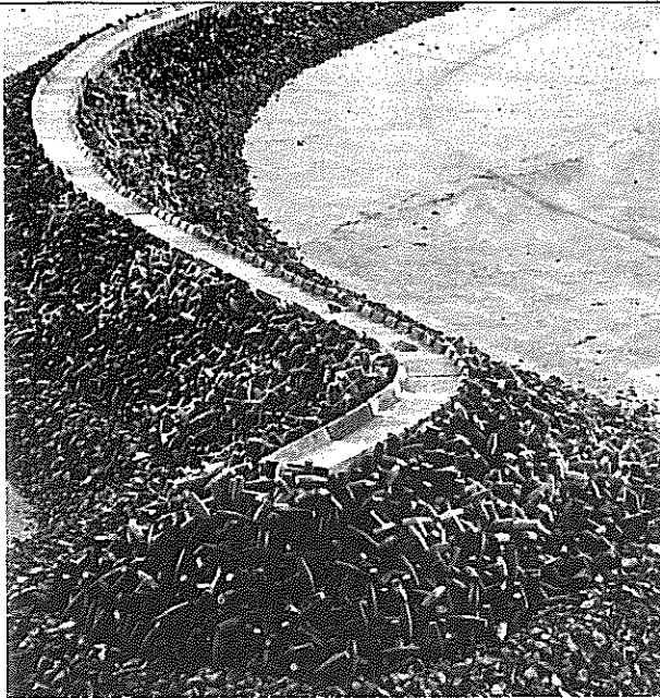
At Stellenbosch the NRIO has at its disposal comprehensive facilities for coastal engineering and hydraulic model studies. Shown in the photograph is a scale model of the proposed south breakwater head for Richards Bay.
