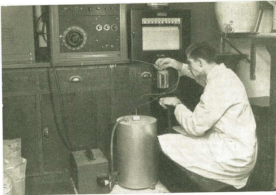
A platinum-wound high temperature furnace being used for weight loss determinations in research on South African clays.
