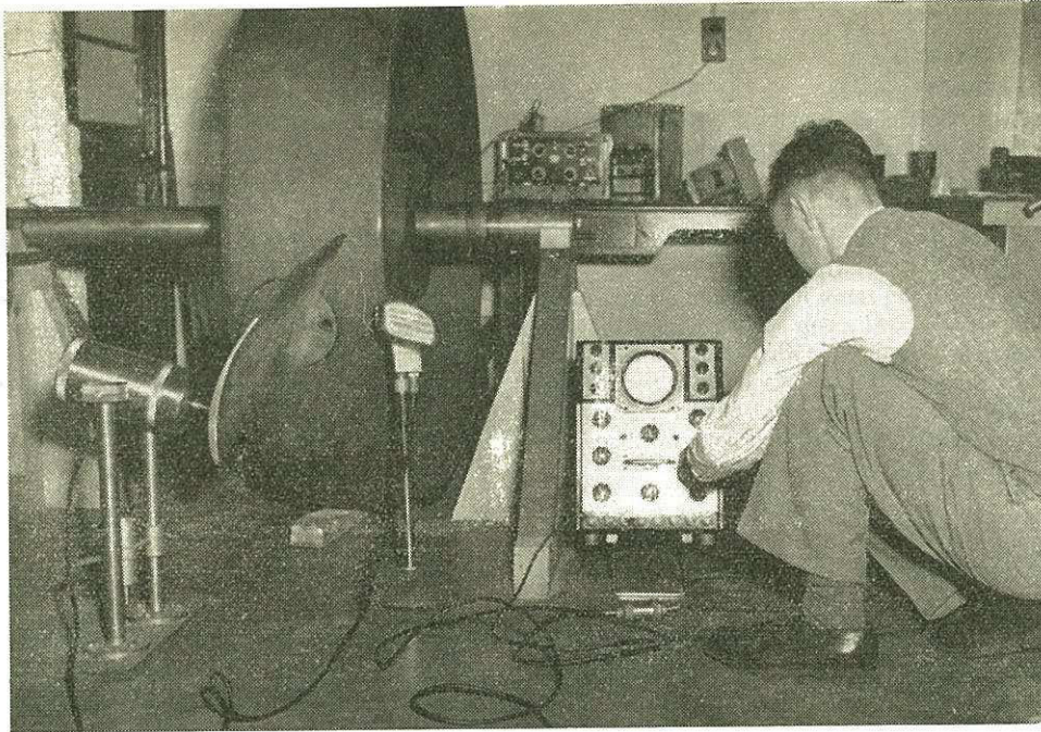
Measurement of the natural frequency of vibration of a fan blade.
