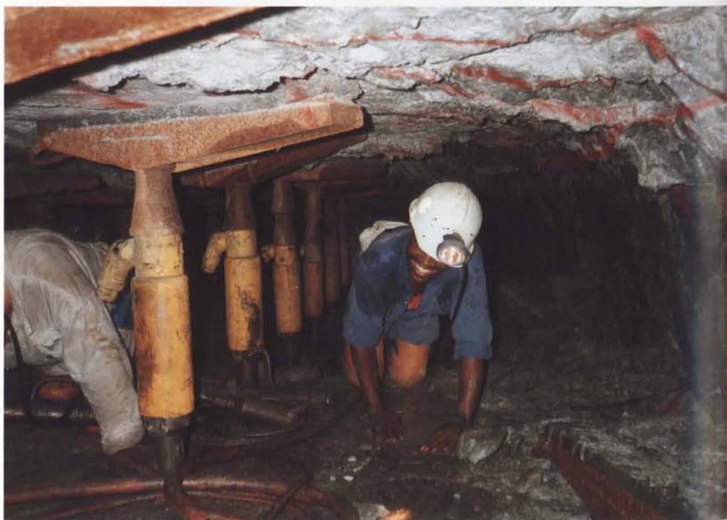
Rapid-yielding hydraulic props which provide improved protection against rockfalls and rockbursts at the stope face in South Africa's numerous deep mines. This development is one of the many assets acquired by the CSIR via its merger with the Chamber of Mines Research Organisation.
