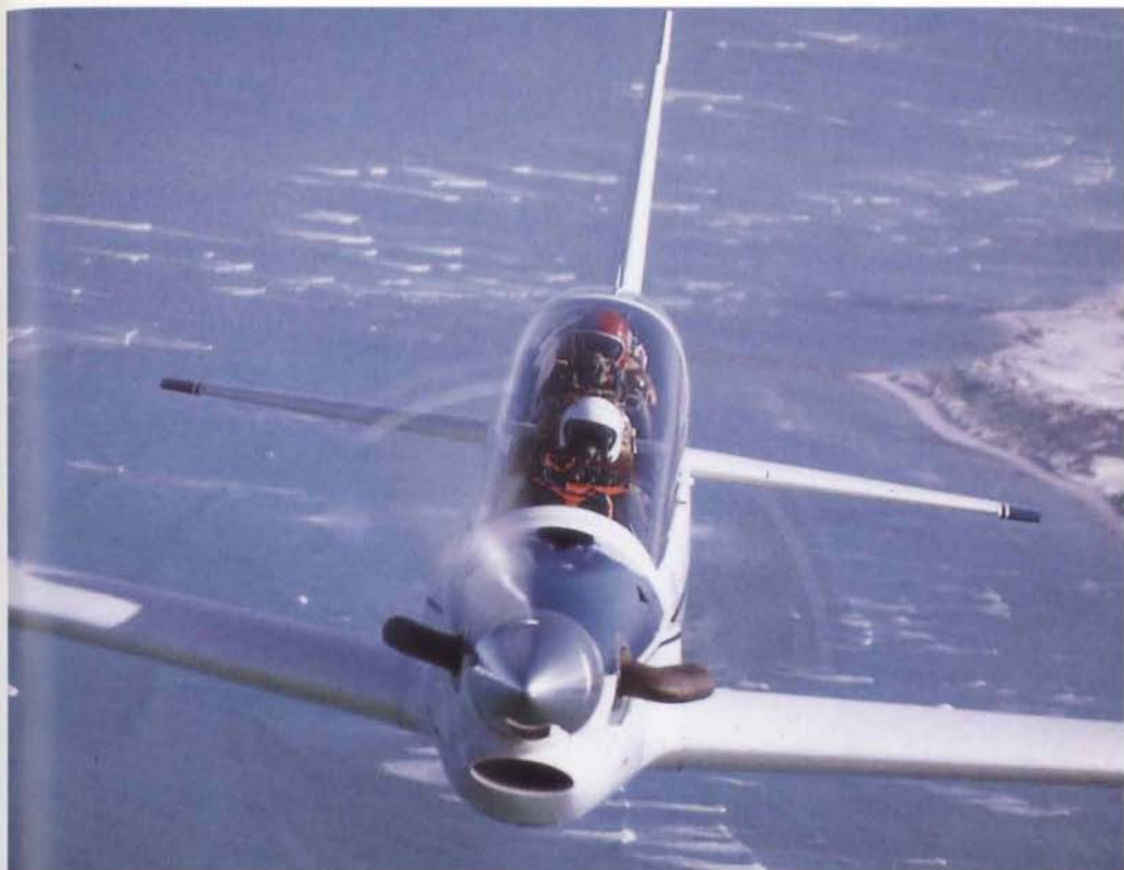
ACE, the CSIR-designed all carbon-fibre turboprop trainer aircraft, previously named OVID. (Nic Papastefanou)
