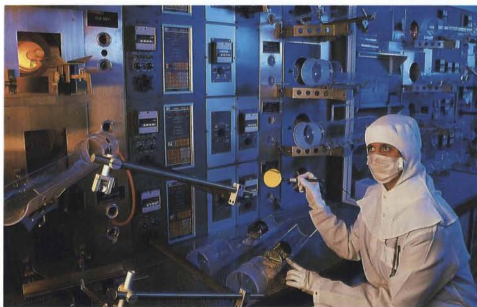
A glowing disc of silicon is taken from a furnace in the IC manufacturing facility of the National Electrical Engineering Research Institute.
