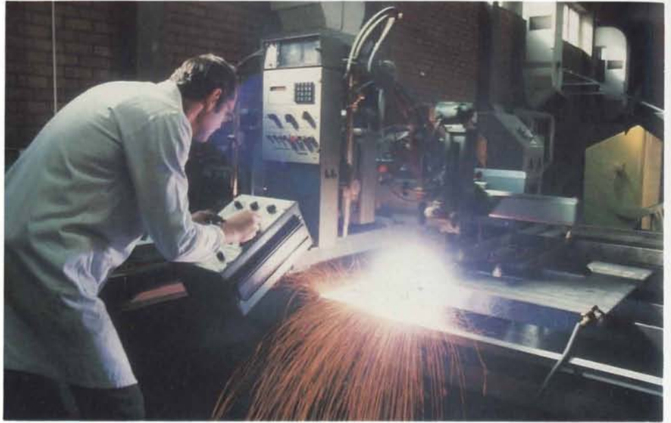
A numerically controlled profile cutting machine in the plate metal workshops of the Technical Services Department.
