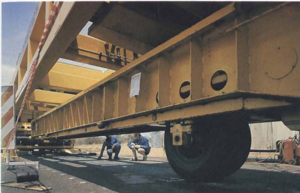
The Heavy Vehicle Simulator developed by the National Institute for Transport and Road Research.
