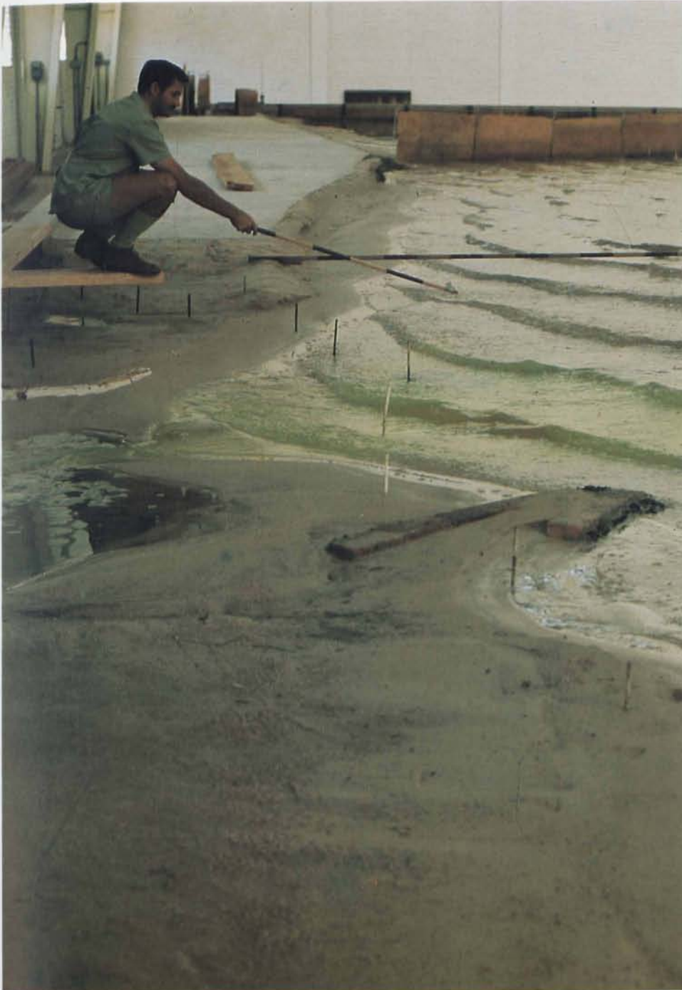
A harbour design is tested in the hydraulics hall of the National Research Institute for Oceanology in Stellenbosch.
