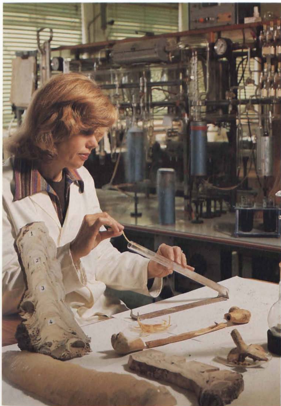
The radio carbon dating facility of the National Physical Research Laboratory. Determining the age and thickness of layers in stalagmites can provide information on past rainfall patterns.
