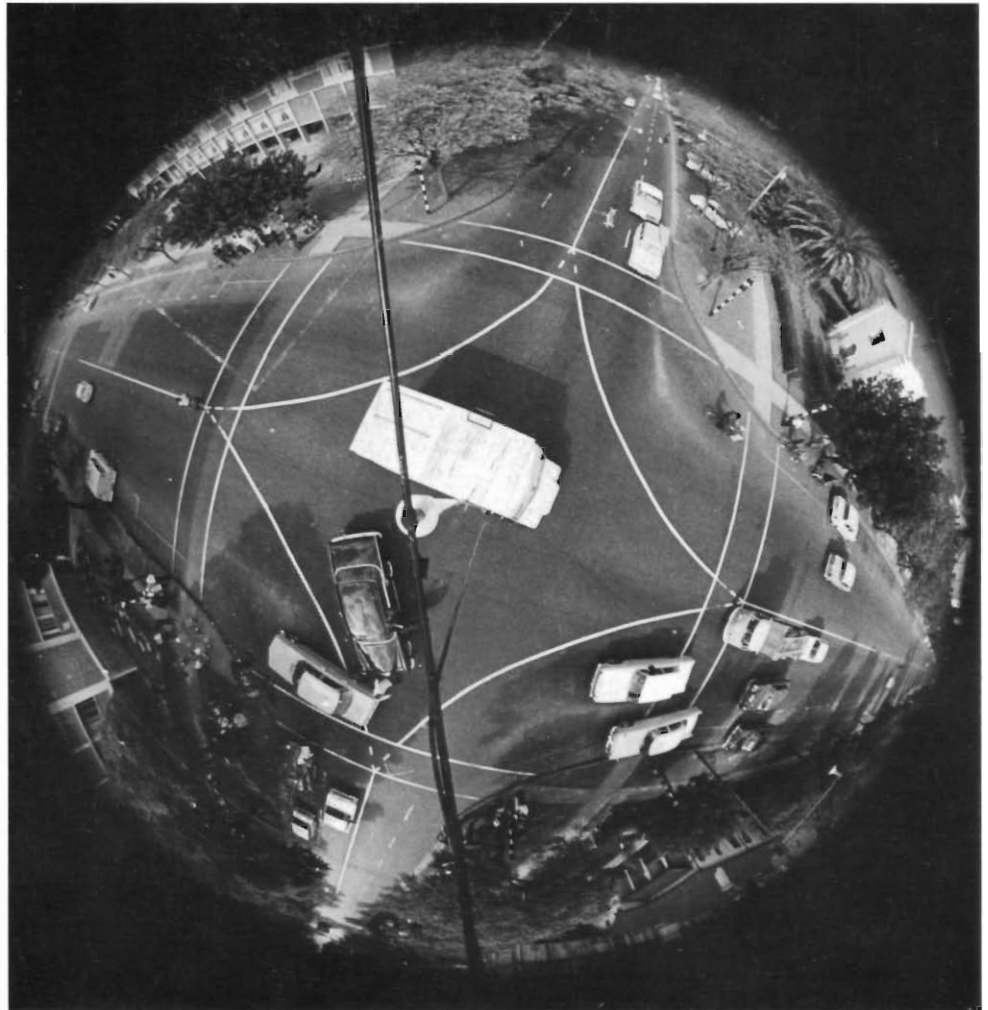
A vertical photograph of a collision scene taken with a 'fish-eye' camera in an on-the-spot investigation by the road accident research team of the National Institute for Transport and Road Research.
