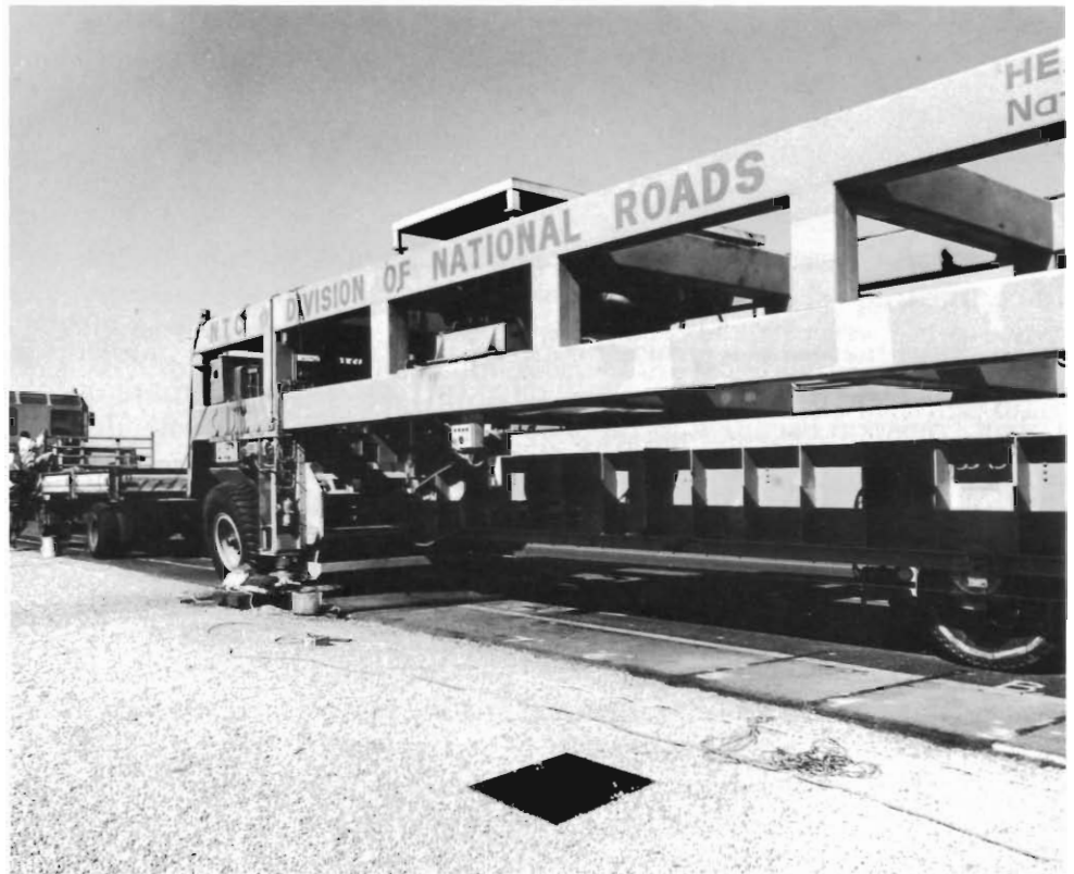
The heavy vehicle simulator developed by the National Institute for Transport and Road Research.
