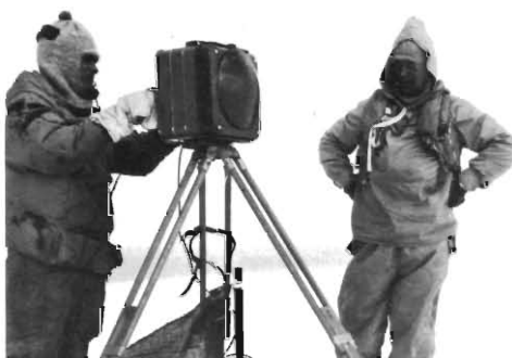
Various models of the Tellurometer system of distance measurement. The bottom right photograph shows Dr Trevor Wadley, inventor, using a recent model with some assistance from a representative of the manufacturing firm, Plessey SA Ltd.
