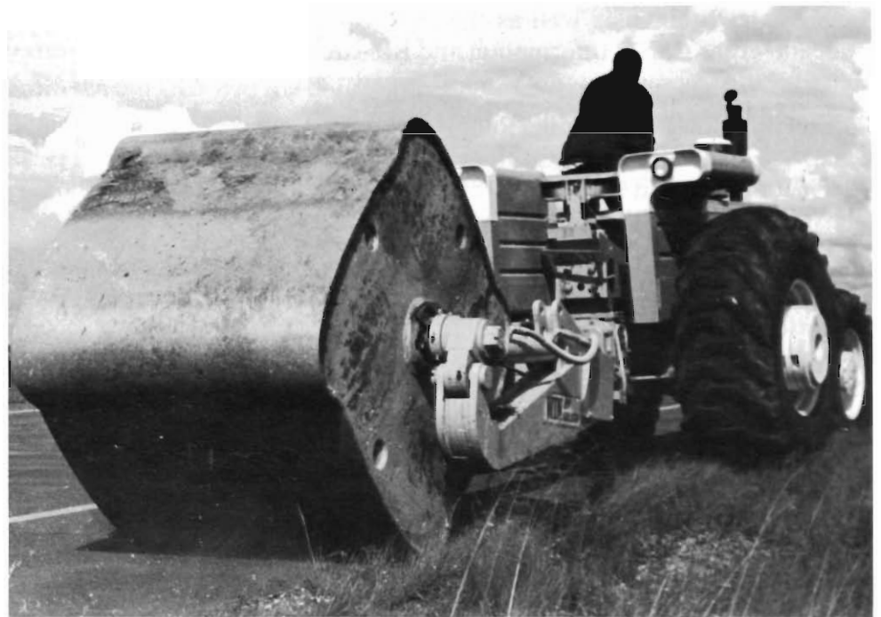
The 'Impact Roller', developed by the National Institute for Transport and Road Research in collaboration with the South African Inventions Development Corporation
