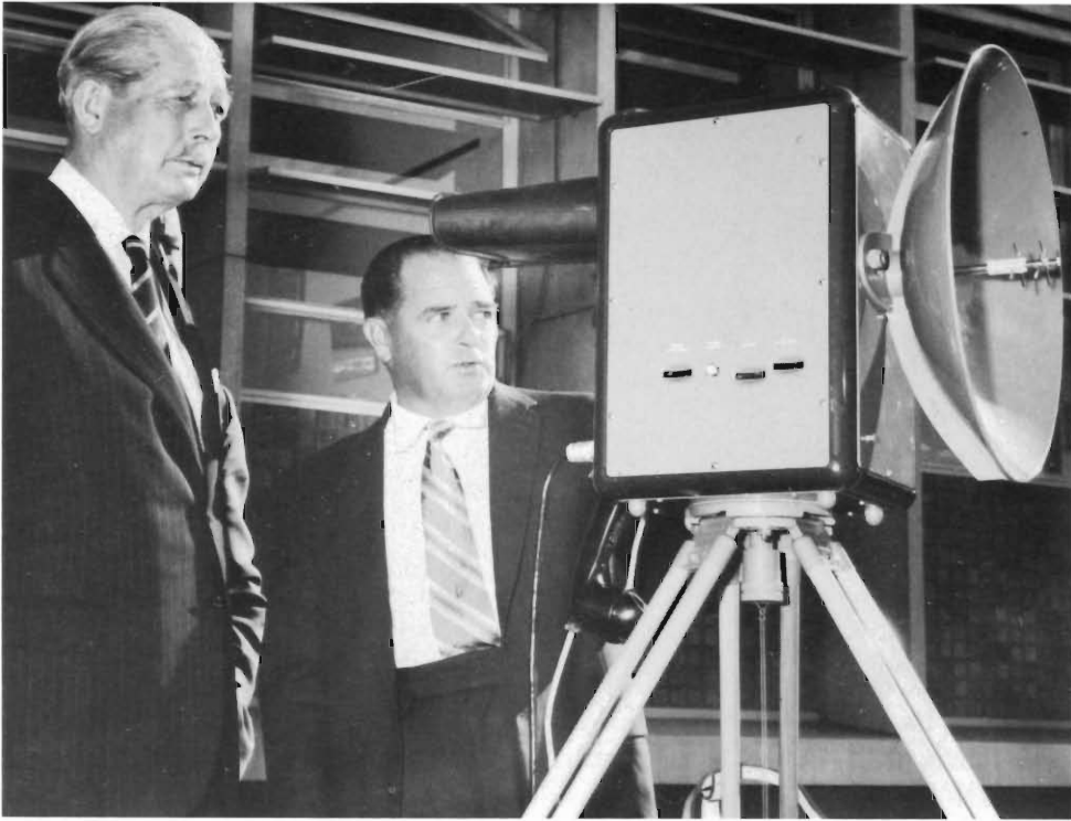
Dr Trevor Wadley demonstrating his 'Tellurometer' distance measuring system to British Prime Minister Sir Harold MacMillan during the latter's historical visit to South Africa in 1960.
