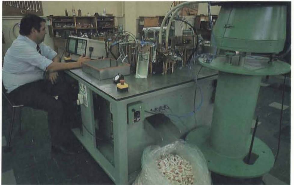
A low-cost automation system for manufacturing lipstick cartridges, developed in the Technical Services Department for a South African industry.
