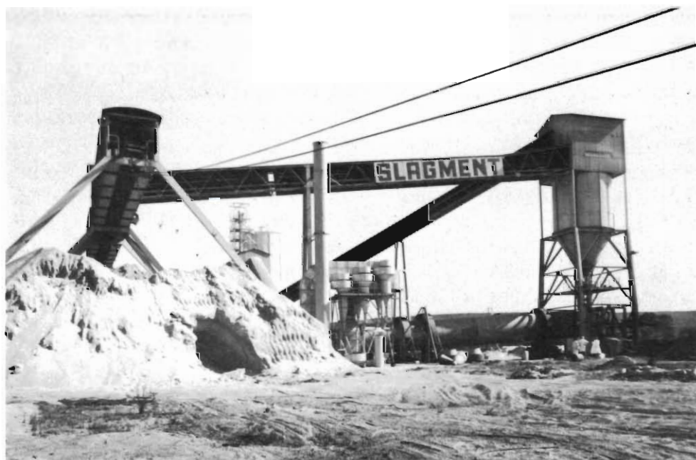
A plant producing slag cement from steelworks slag with a high magnesia content.
