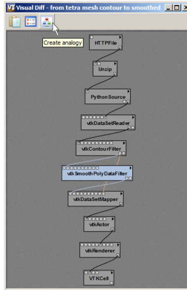
Figure 9.4: Click the Create Analogy button in the Visual Diff window to create a named analogy.
