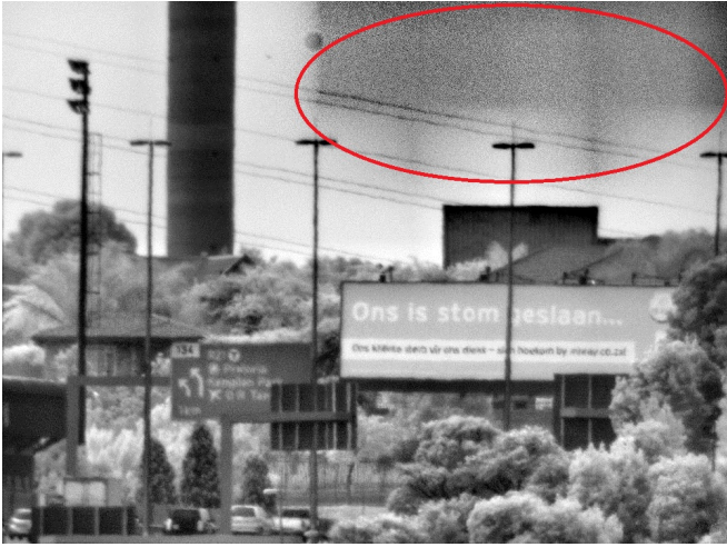
Fig. 3. Result after applying the adaptive \alpha and \beta values to the MSR image of the Road input image which can be seen in figure Fig.7. The indicated region shows the over-gain problem experienced in areas of the image where the image intensities are very uniform.
