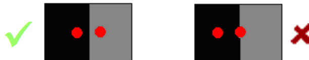
Fig. A1.11. Illustration of how to position the two spots on the SLM.
