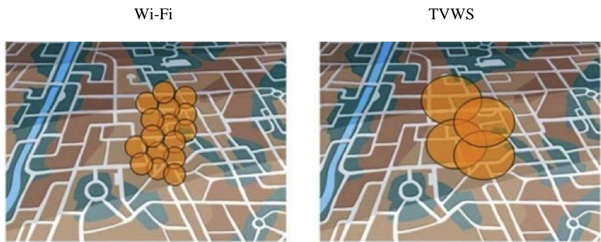
Figure 1: A coverage comparison of traditional Wi-Fi AP to that of CRs over TVWS [9].
