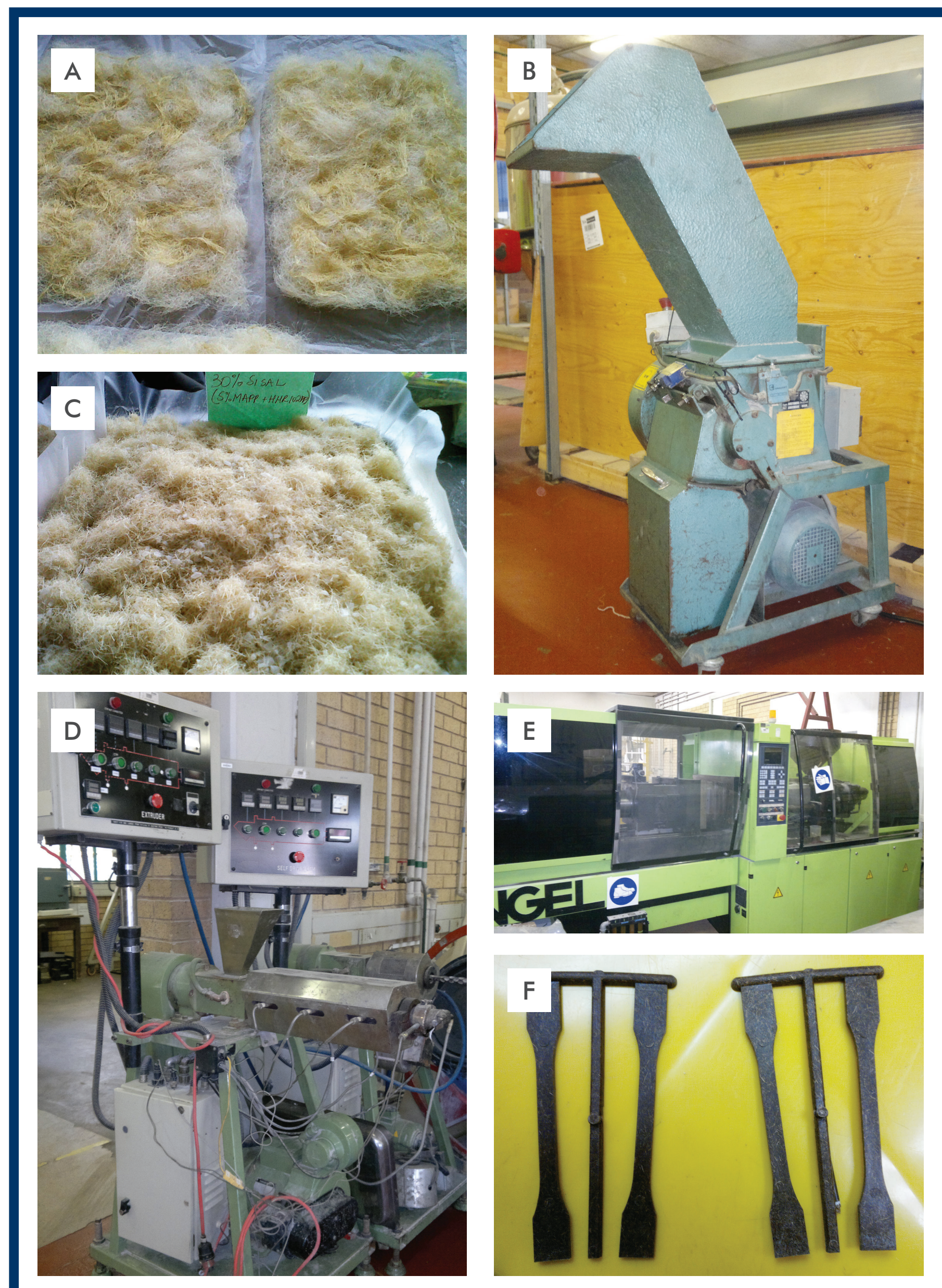
(B) High speed granulator, (C) Composite granules, (D) Single screw extruder, (E) Injection moulder and (F) Composite samples (dumbbells)
