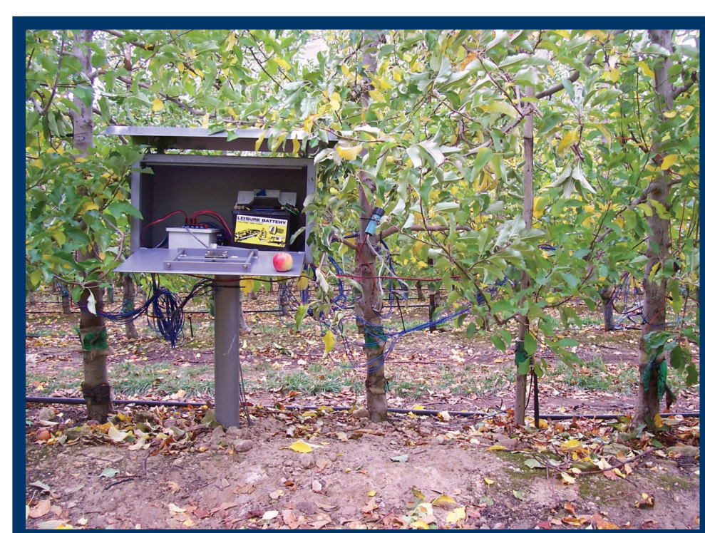
Figure 1: Heat Pulse Velocity system used to measure sap flow (transpiration) in the apple orchard
