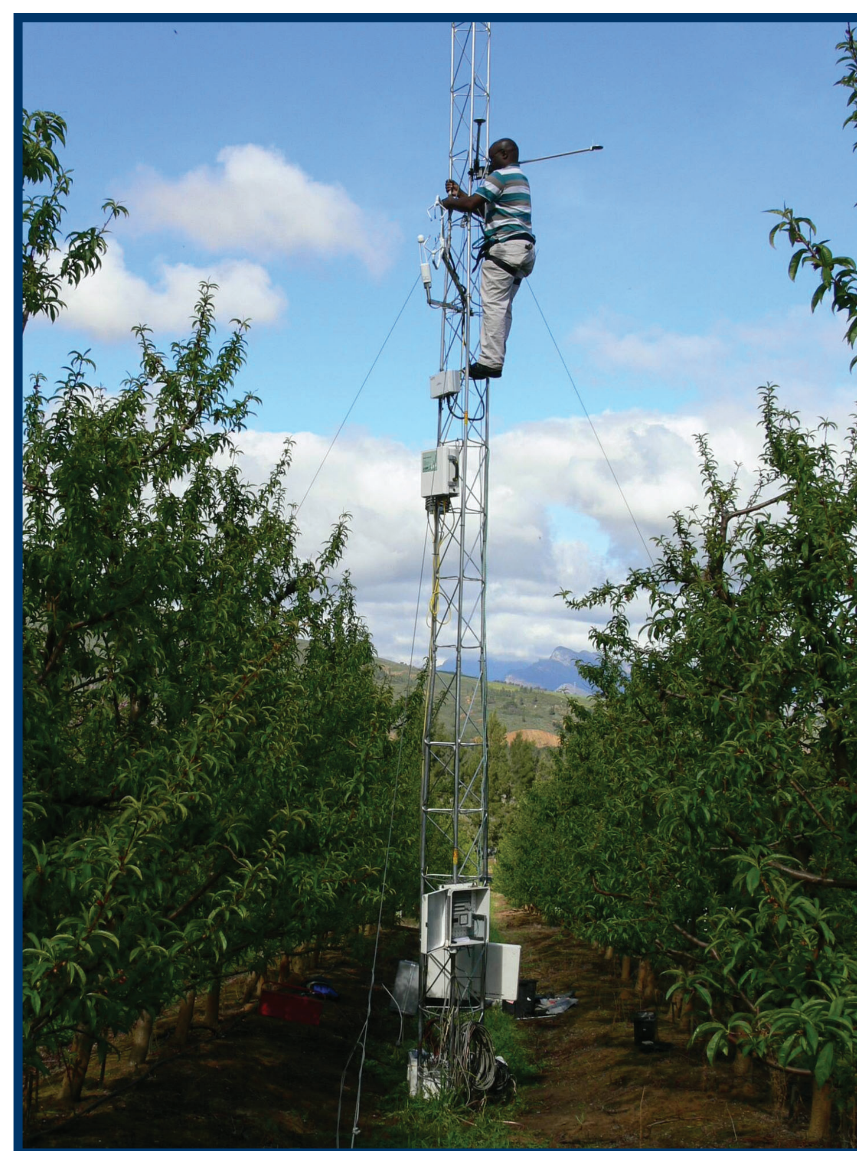
Figure 2: Open path Eddy Covariance system mounted on a lattice mast, and used to measure total evaporation in the nectarine orchard.
