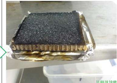
Surface of panel showing exfoliated vermiculite and protective char layer
