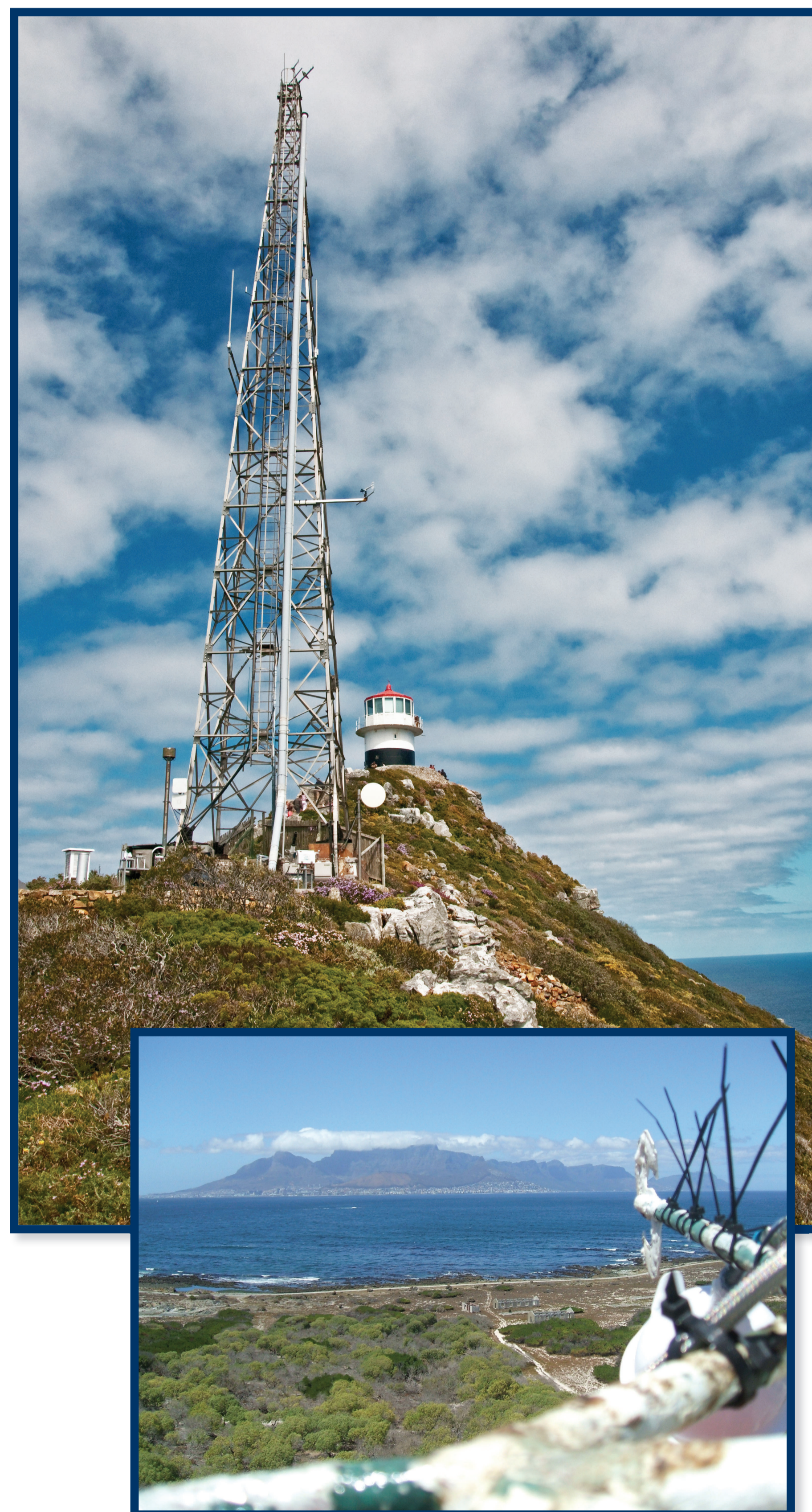
Figure 2: The main wind directions across the Cape Town metropolitan area are from the northwest and southeast. By placing monitors at the lighthouses at Cape Hangklip and Robben Island, it is possible to measure clean maritime air on the upwind side of the city, and polluted air downwind, for both of these wind directions. The monitor at Cape Point allows north easterly winds to be monitored as well. It also provides globally-important information about sources and sinks in the vast South Atlantic Ocean
