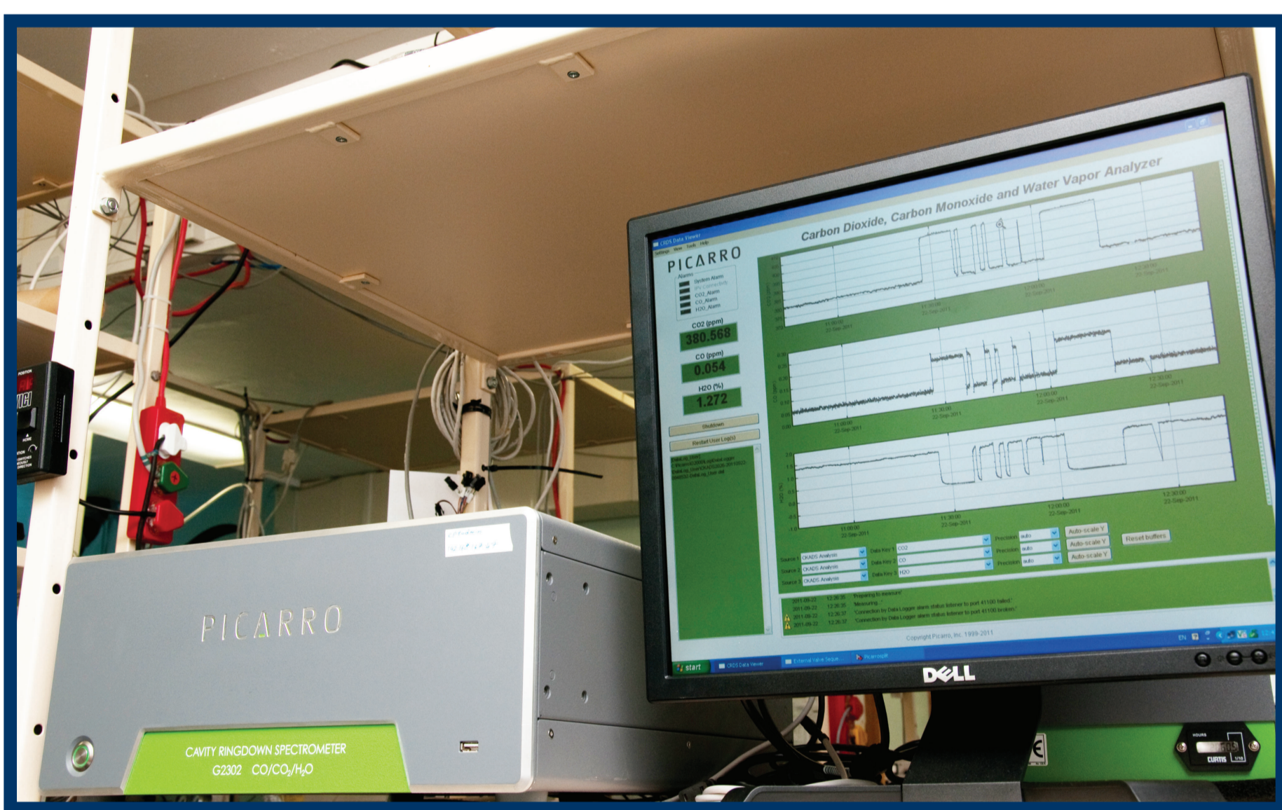
Figure 1: The Picarro Cavity Ring-Down spectrometer provides very precise and stable measurements of several greenhouse gases. To ensure that all the instruments in the system are exactly calibrated, they are checked on a frequent basis against test gases provided by the National Oceans and Atmosphere Administration in the USA
