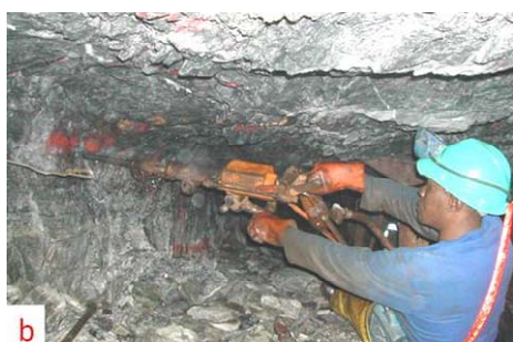
(b) Drilling a stope face underground in the Free State gold field.
