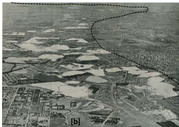
(b) Photo of Witwatersrand showing outcrop (dotted black line) of reef in Central Rand area (Jeppe, 1946a).
