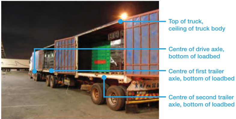
Figure 26: Location of accelerometers on trucks
