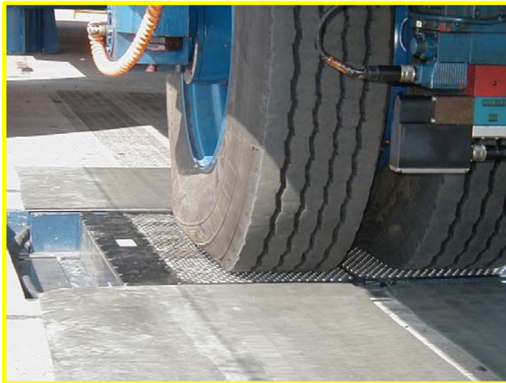
FIG. 13. Dual SIM device under tire loading using the Heavy Vehicle Simulator (HVS).
