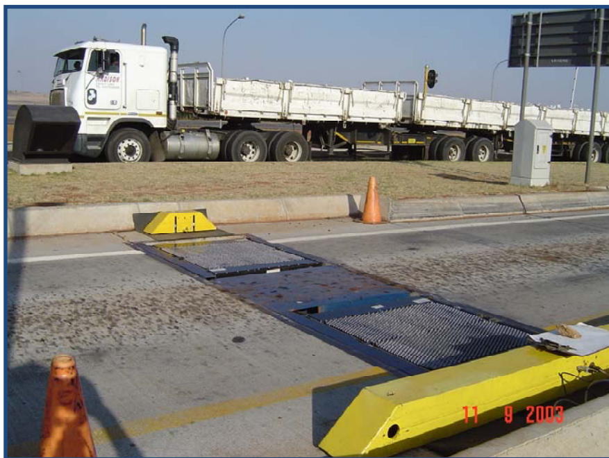
FIG. 20. Typical field configuration during a special test series with a quad SIM system conducted in 2003 in South Africa at the Heidelberg Traffic Control Center.
