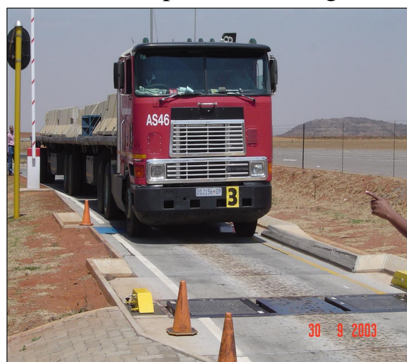
Four-pad Stress-In-Motion (SIM) system used for tyre mass data
