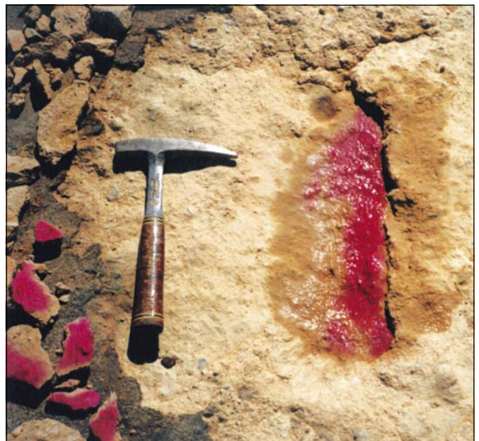
Photo 7 Roller-induced shear plane dipping to right with overturned shear "biscuits" (uncarbonated on lower surface) lying at left. Loose to very weak (could be broomed or easily scratched off) to 20 mm, and carbonated and weak to 40 mm below top of primed, 3% cement-stabilised, weathered granite base. Detected by chain drag
