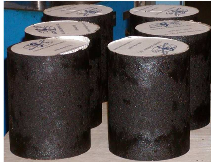
Gyratory Compacted – Modulus/Deformation Tests
