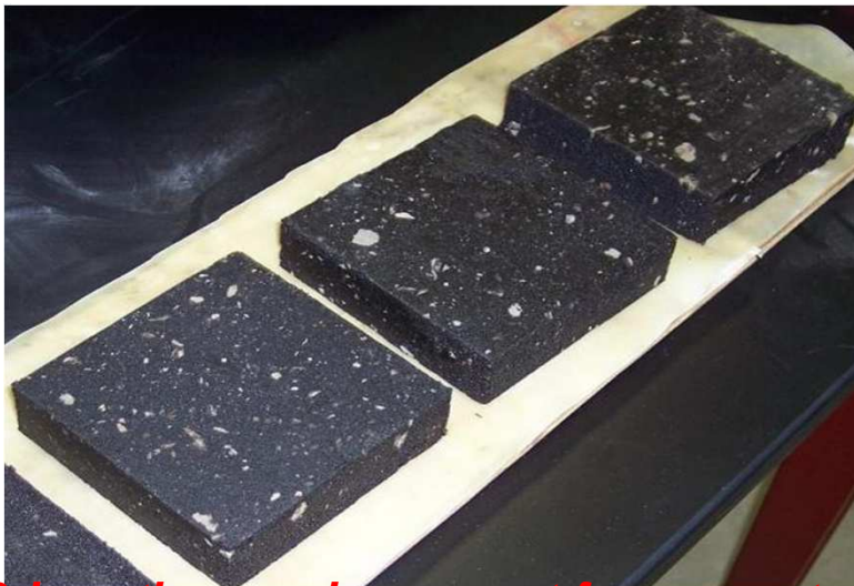
Prismatic specimens cut from gyratory compacted specimens – Direct Shear Test
