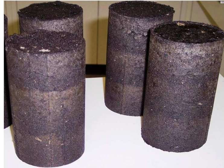
Standard Proctor Compacted – Shear Test
