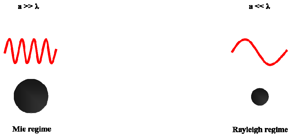
Figure 1.3: In the Mie regime the diameter of the particle to be manipulated is large compared to the wavelength of the tweezing beam and in the Rayleigh regime the particle is much smaller than the wavelength of light used for tweezing.
