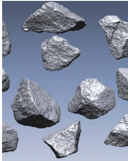
Actual aggregate particles (left) and scanned and processed particles of a typical South African asphalt mix.
