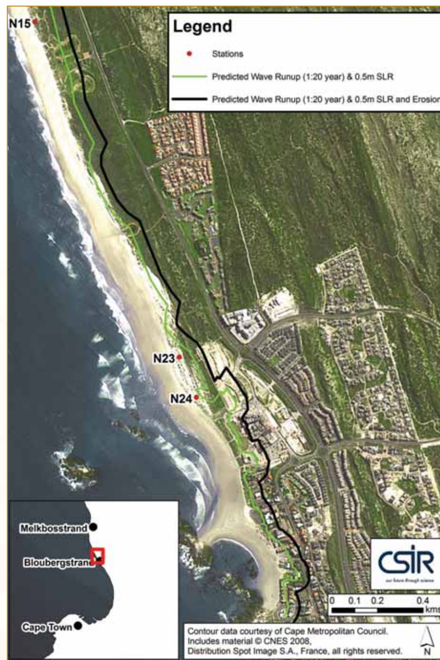
Map 8.6. Illustration of predicted combined effects of potential shoreline erosion with Bruun's rule and higher wave runup for a 0.5 m rise in sea level and a 1-in-20-year sea storm on the Blaauberg coast. Source: Theron, Diedericks, Maherry and Rossouw, CSIR (2010).
