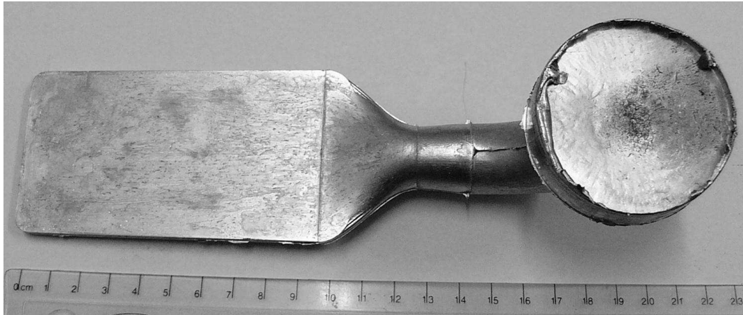
Figure 2. The actual semi-solid rheocast high purity aluminium plate (including the runner and biscuit)
