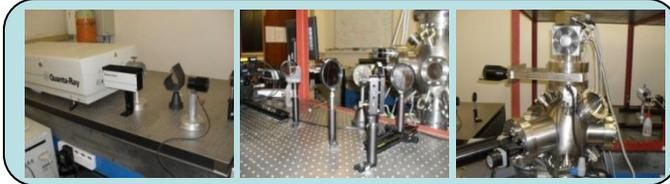
Fig 1: The Nd:YAG laser, optical set up and the PLD chamber used in this study
