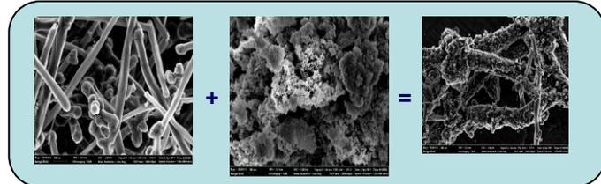
Fig 3: SEM micrographs showing the MWCNTs, NiO powder and the coating of the MWCNTs with NiO in the composite thin film
