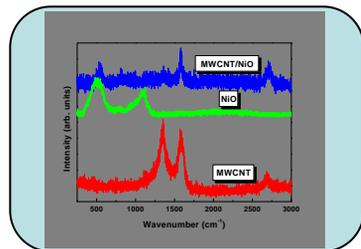
Fig 4: Comparison of the Raman spectra for MWCNT, NiO and the MWCNT/NiO composite
