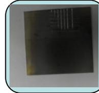
An ISO scratch test was carried out to determine the strength of adhesion of the thin films onto the aluminium substrates. The scratch test measures, on a scale of 0 – 5, how much material has been removed from the substrate. Shown on the left is a picture of a sample that has been scratched. This sample was given a score of 0.5, showing that very little to no material was removed indicating that the PLD technique of depositing SSA material passes this scratch test.
