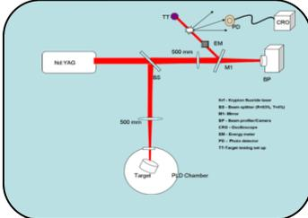
Fig 1 above (from left to right), shows the Nd:YAG laser, the optical set up and the Pulsed Laser Deposition chamber (PLD). Fig 2 shows the schematic diagram of the experimental set up. The Laser used is a Quanta Pro series Nd:YAG, which is capable of delivering four wavelengths: 1064, 532, 355 and currently operating at 266 nm. The energy per pulse for the work reported is 60 mJ and the beam intensity is 2 mJ/cm<sup>2</sup>. The repetition rate is 10 Hz.
